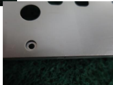
Laser Welding No mark on another side after 2 parts firmly welded
