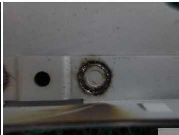
Laser Welding No mark on another side after 2 parts firmly welded
